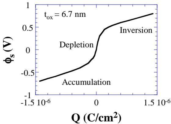
Fig. 4 Surface potential versus surface charge. After Roy et al.<sup>25</sup>
