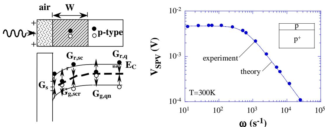
Fig. 3 Sample geometry and conductances due to generation and recombination of excess carriers and experimental/theoretical surface photovoltage data.<sup>17</sup>
