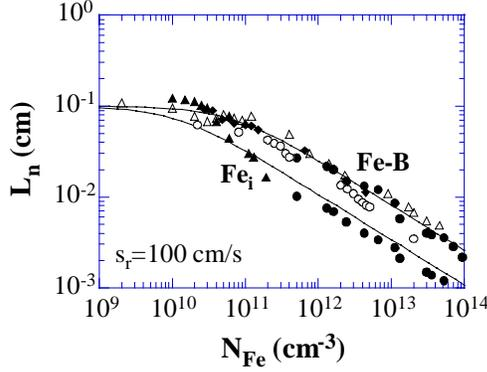
Fig. 2 Effective minority carrier diffusion length for  $Fe-B$  and  $Fe_i$ . The flattening of the data at low iron densities is due to surface recombination. The solid lines are calculated with a surface recombination velocity of 100 cm/s.
