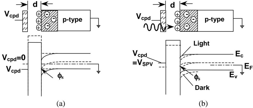
Fig. 1 Surface voltage probe energy band diagram: (a) dark and (b) optical excitation.
