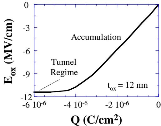
Fig. 5 Oxide electric field versus surface charge for an oxidized wafer. After Roy et al.<sup>25</sup>
